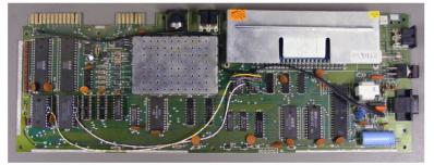
This stage allows for an intermediary check: If you switch on your VIC without any hardware expansions, you should now already see '6655 BYTES FREE'. Even though, to complete part 2 of the mod, a small modification needs to be done on the solder side, to ensure that cartridges in the expansion port can't make trouble. Stay tuned.
